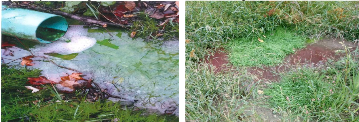
Figure 6: Dye test showing illicit discharges to waters of the state during HSTS evaluation
